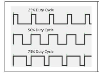
As it can be seen in this image, PWM is basically a square wage signal, of a chosen frequency, where only the duty cycle is varied from 0% to 100%, in order to control the amount of energy delivered to a load.
