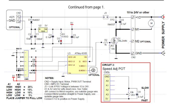
The circuit diagram above illustrates all the components and circuitry of the PWM speed controleer. The top left-hand-side of the diagram (U2) shows the regulator that provides the 5V required to supply the microcontroller (U3) just below the regulators.
