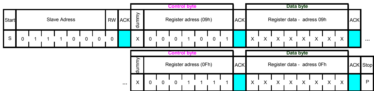
Figure 15: I 2 C multiple write protocol
