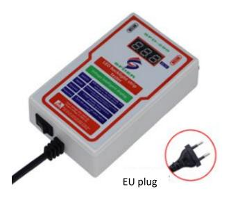
Input voltage: 85-265V (international general), output voltage: 0-300V, power 25W.Automatic detection of output voltage and output current. Can test any size LED backlight and lamp bead. High brightness, no need to dismantle the screen that you can judge the backlight.
