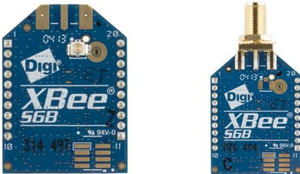
XBee WiFi modules with a U.FL (left) and SMA (right) antenna connector.
