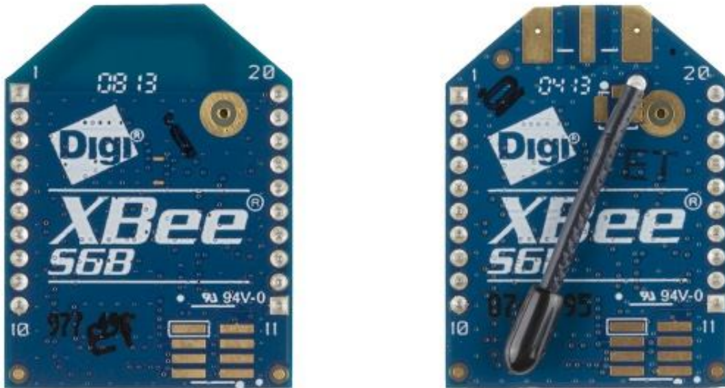
XBee WiFi modules with PCB antenna (left) and whip antenna (right). No external antenna needed!
