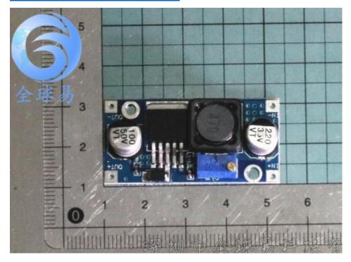
The XL6009/**XL6019** is a high performance BOOST (BOOST) module with 4A switching current. The module uses XL6009E1/XL6019E1 of the second generation of high-frequency switching technology as the core chip, and the performance is far superior to that of LM2577 of the generation technology. The XL6009/XL6019 booster module has lower cost and better performance, and the LM2577 module is about to be phased out.
