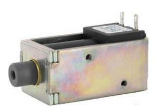
Stroke: 7 mm Force at beginning of stroke (FM: 100/25/5%): 4/3/3 N Force at end of stroke (FM: 100/25/5%): 10/6/5 N Power Consumption (FM: 100/25/5%): 12/44/200 W Total mass: 300 g Degree of protection / Energetic class: IP 40 / B Standard supplies: 24Vcc Possibles supplies: From 12 to 220Vcc Duty Cycle: Permanent, impulsions (100 / 40 / 25 / 15 / 5 %) Standard: NF C 79300 Examples of applications: Automatons, electrical equipment, machinery, security applications.
