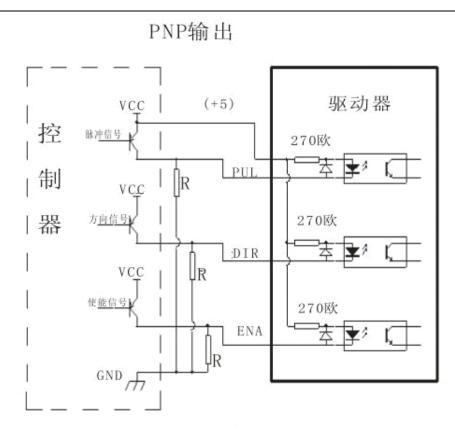
Note: When VCC=5V, R=0 When VCC=12V, R=1K, >1/8W When VCC=24V, R=2K,>1/8W
