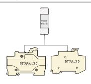
Matched schematic diagram of fuse protector supporter (pedestal) and fuse links with size of  $14 \times 51$
